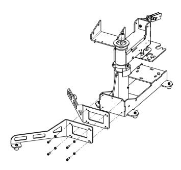
• Connect the press lever to the frame of the TS5E using screws and washers.
