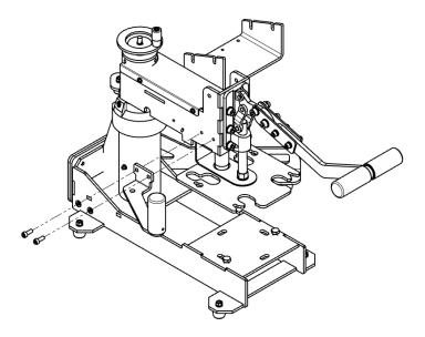
• Lift the base plate over the frame of the TS5E and thread the screw heads of the hexagonal screws through the keyhole milled holes on the adapter plate on the underside of the base plate. (For simplicity, the illustration shows only the adapter). Slide the base plate in the direction of the arrow until it touches the screws and tighten the screws.
