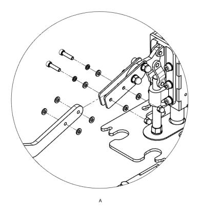
• Now attach the swivel handle as shown in the illustration. Use the two M6x16 mm screws and the two M6 washers for this. After this step you can remove the cable tie so that you can swing the heat press open.
