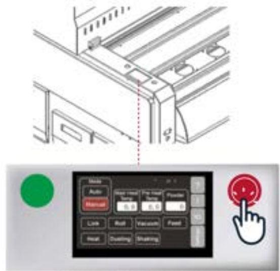
Press to activate. Rotate the button to the right to exit the emergency stop state
